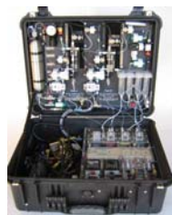
Figure 3. The InnovaPrep hydrosol concentrator used to concentrate surface sample extracts collected during this testing.
